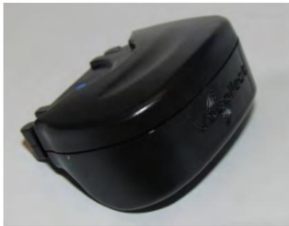
図 113 : SRX2 Wireless Headset High-Performance Battery
