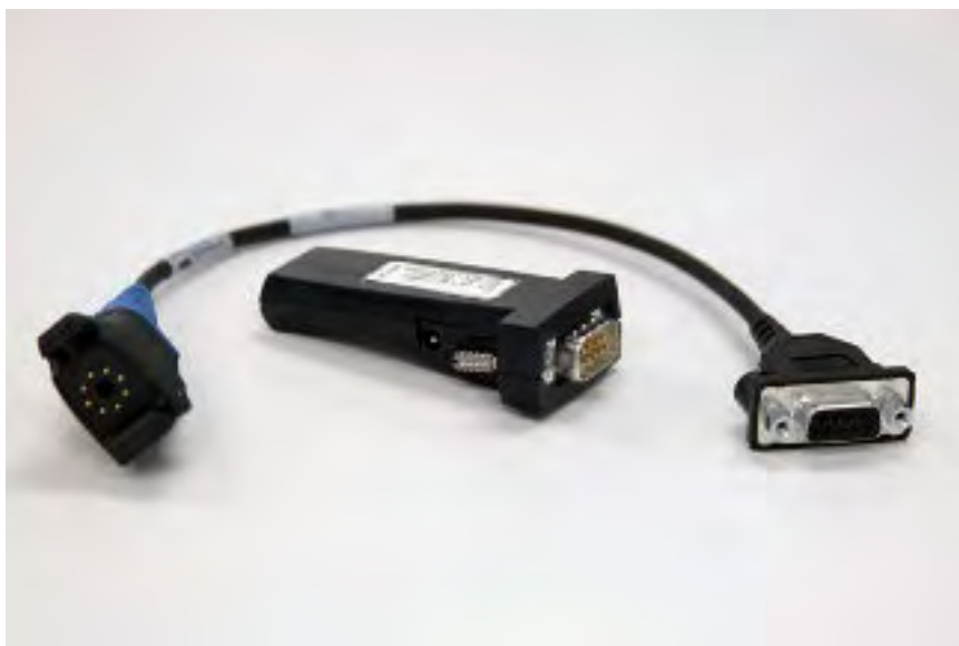
Figura 85: T2x Bluetooth Serial Adapter
