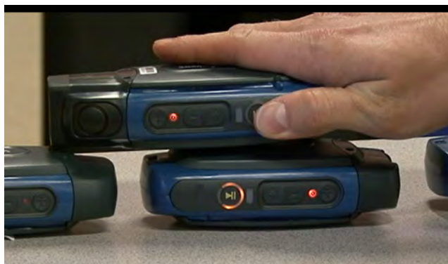
Figure 4: Transferring the Configuration Using TouchConfig
