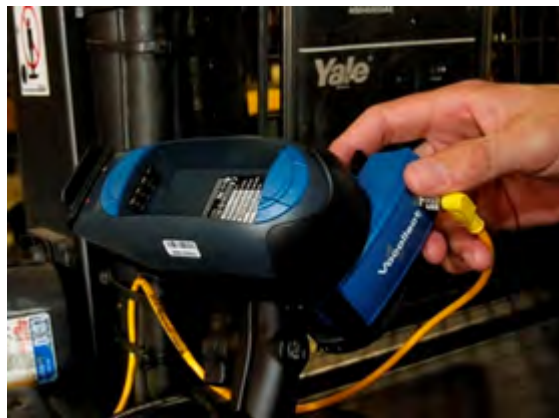
Figure 19: Battery adapter docked in VMT configuration
