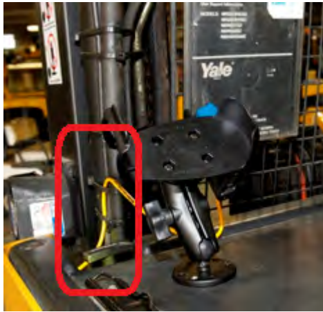
Figure 22: Cables secured on a vehicle
