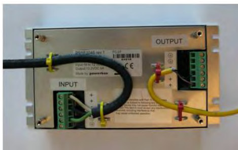
Figure 16: Cables Attached to the Power Supply
