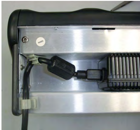
Figure 25: Cable Routed Through Plastic Clips
