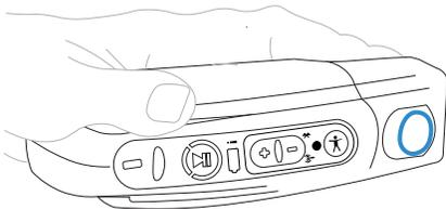
4. Direct the lighted aiming frame so that it completely contains the bar code.
