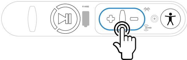
The device says "faster" each time you press the + button and "slower" each time you press the – button. If the speed of the voice is at the fastest possible setting, the device says "This is fastest." If the speed of the voice is at the slowest possible setting, it says "This is slowest."
