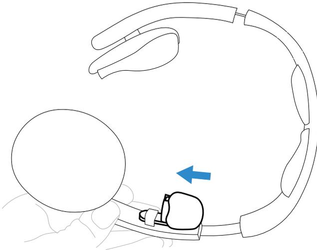
3. Remove the electronics module from the headband.
