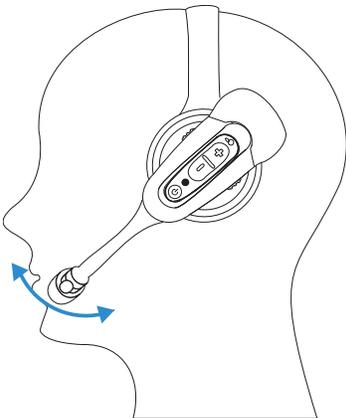
5. Make final adjustments with the flexible boom so that the microphone is positioned correctly. Position the microphone as close to your mouth as possible, but outside of your breath stream. It should be facing your upper lip, and not touching anything (for example, clothing, skin, or facial hair).
