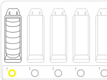
6. When the ring LED indicator turns a solid green, the battery is fully charged. Pull the battery off the charger port to insert it into the device.
