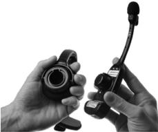
3. Push the electronic module into the hub pocket until it is firmly seated.
