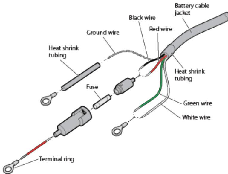
5. Insert and secure the fuse in the fuse holder assembly.
