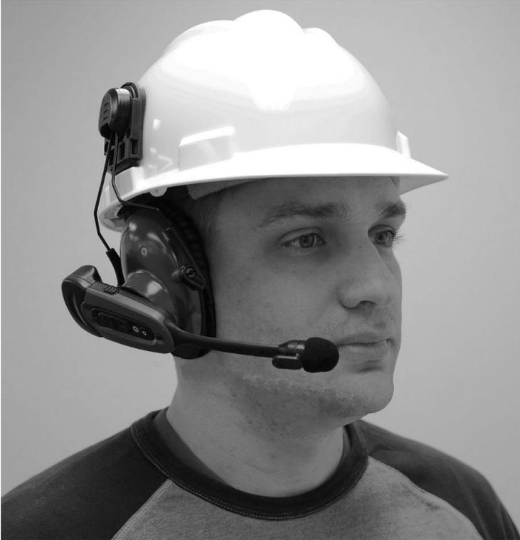
When using the TouchConnect™ feature to pair the SRX2/SRX3 Hard Hat Headset with a Talkman A700/A700x Series device, you can obtain the operator ID by touching the device to the
