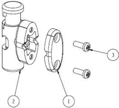
4. Insert the supplied screws (3) through the holes in clip assembly part 1 and into part 2.
