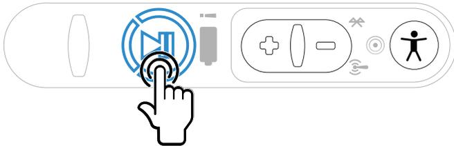
1. Press the **Operator** button. The device says "Current operator is **operator name**. Select menu item."
