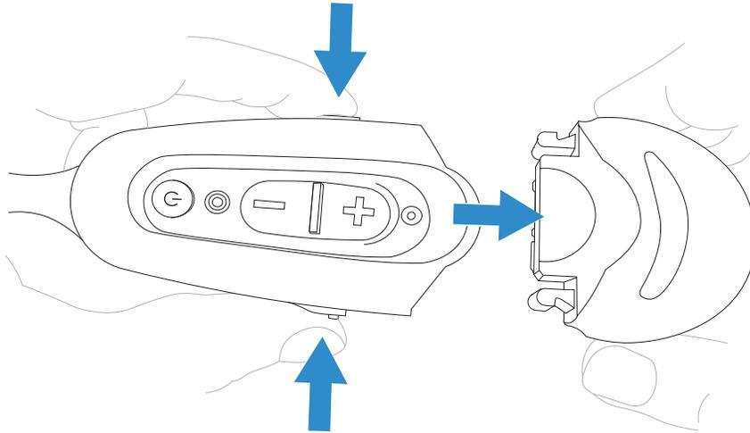
3. With your other hand, hold the battery at the end of the electronic module opposite the mic boom.
