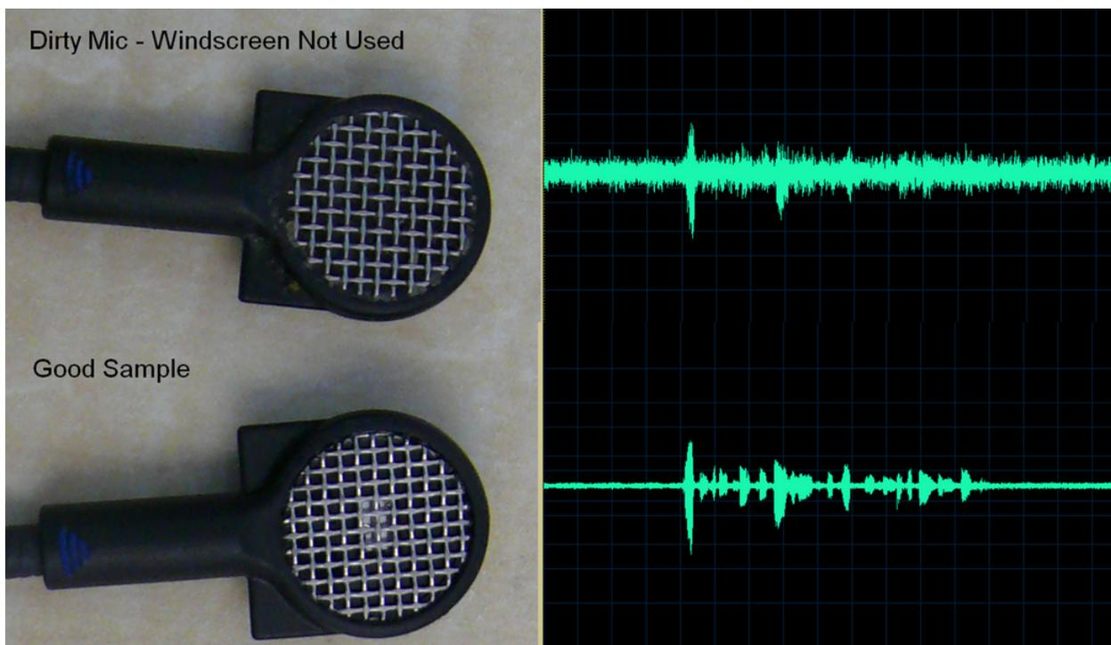
The comparison shows how an unprotected microphone cannot make clear distinctions between speech and silence, while a clean microphone can.
