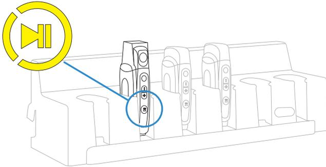
5. When the device battery is charged, the device state indicator is lit green.
