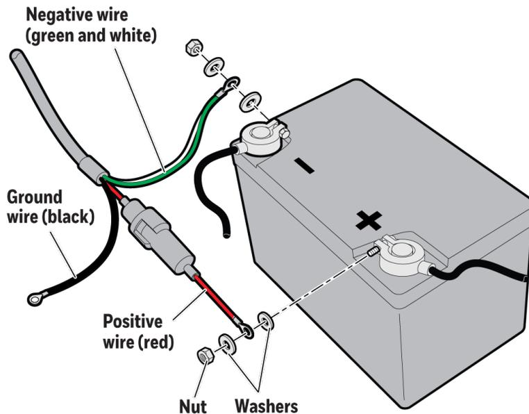
2. Place a 3/8-inch washer onto each end of the battery clamp bolt.
