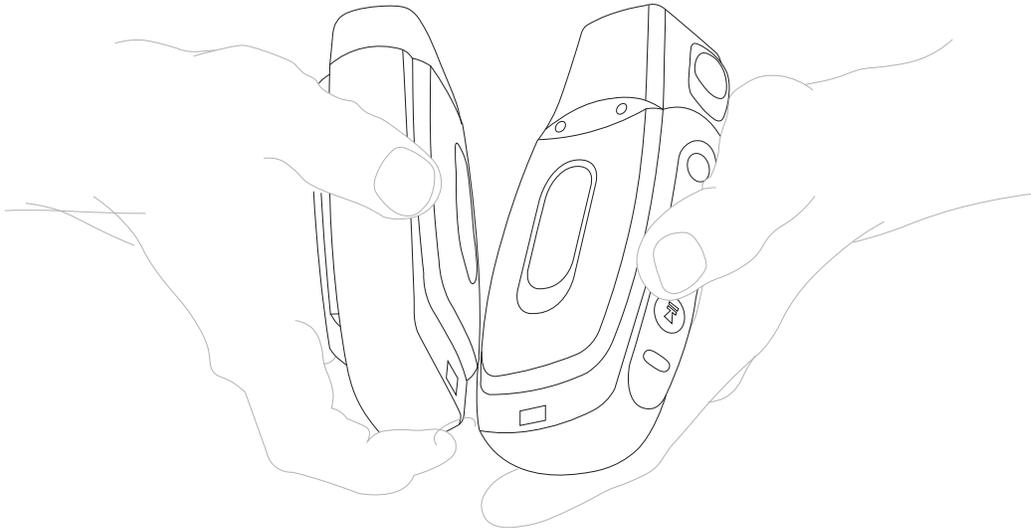
6. Watch the device state LED indicator ring on the receiving device to confirm configuration success or failure.
