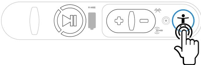
The device says "higher" each time you press the + button and "lower" each time you press the – button. If the pitch of the voice is at the highest possible setting, it says "This is highest." If the pitch of the voice is at the lowest possible setting, it says "This is lowest."
