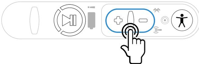
The device says "louder" when the + button is pressed and "softer" when the – button is pressed. If the volume of the voice is at the loudest possible setting, it says, "This is loudest." If the volume of the voice is at the softest possible setting, it says, "This is softest."
