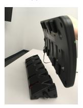
3. Attach the headband rest to the charger by pulling it in opposite directions and aligning the rest with the groves and the holes in the dock assembly. The curve of the headband rest should match the curve of the charger in both configurations.
