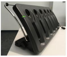
4. Plug the power supply into the outlet and make sure the LED indicator light turns on.
