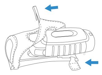
Open Velcro® and slide device out
